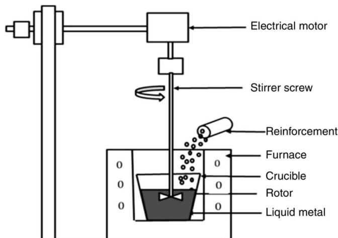
Fig 1: Stir casting setup
