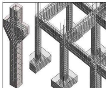
Fig 3: Flanged Concrete Column
