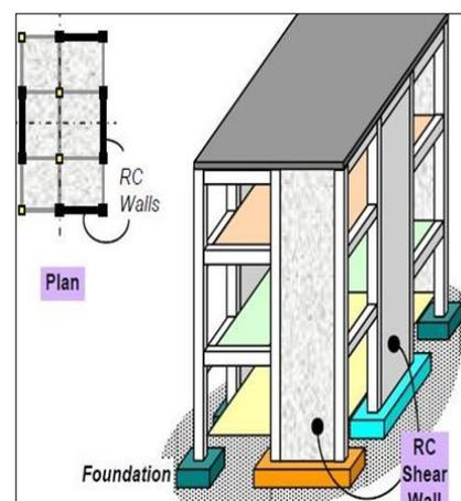
Fig 1: Reinforced Concrete Shear Wall
