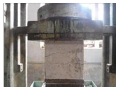
**Fig 1:** Compressive strength test
