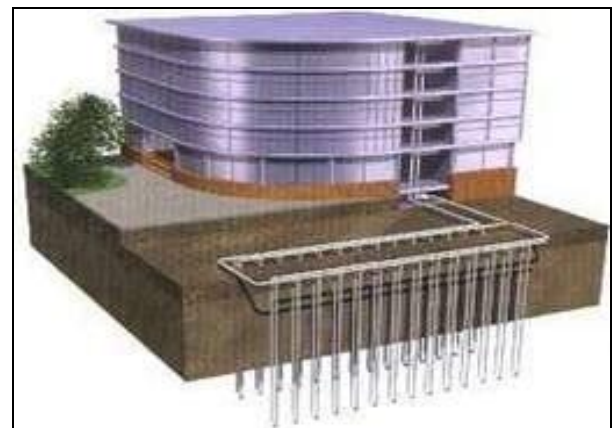
Fig 5: Thermal Stabilization of Soil
