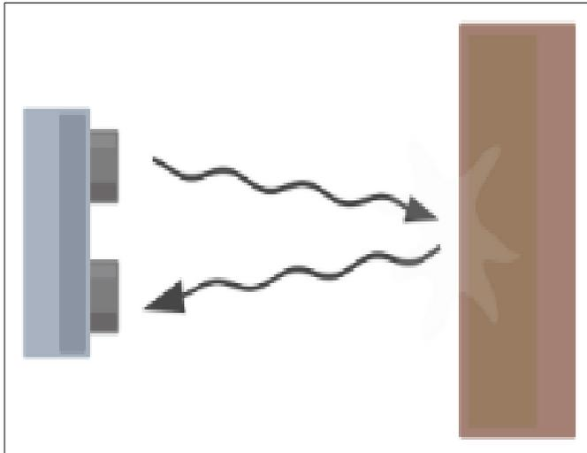
Fig 4: Ultrasonic Sensor Operation
